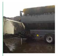
Double sided unrestricted drum access via two large swing out doors allows for easy maintenance and cleaning
