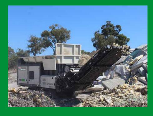
Key features include the hydrostatic drive offering better protection against contamination and allowing for bi-directional shredding. The double shaft shredder has 2m long shafts with a fully welded tooth configuration, impressive throughput and excellent reduction.
