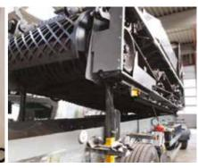
The chassis which can be lifted at the press of a button:
